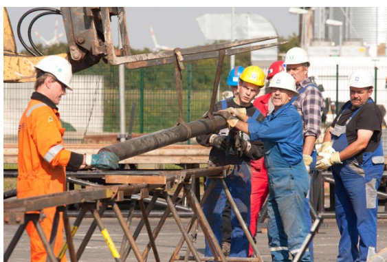
Taking a rock core out of the well Ktzi 203 (Source: GFZ).
