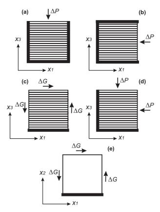
**Figure 1.** Oscillatory tests performed to obtain  $p_{33}$  (a),  $p_{11}$  (b),  $p_{55}$  (c),  $p_{13}$  (d) and  $p_{66}$  (e). The orientation of the layers and the directions of the applied stresses are indicated. The thick black lines at the edges indicate rigid boundary conditions (zero displacements).
