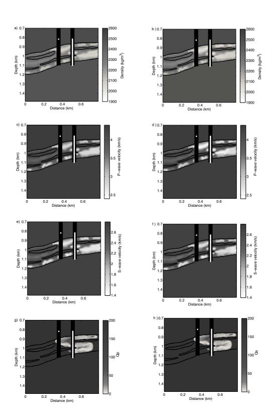
Fig. 11 Panels (a), (c), and (e) show the density, P-wave velocity and S-wave velocity before CO<sub>2</sub> injection, respectively. Panels (b), (d) and (f) show the same properties after CO<sub>2</sub> injection. Panels (g) and (h) show  $Q_P$  and  $Q_S$  at  $f_0$ , respectively, obtained from equation (4), after CO<sub>2</sub> injection ( $Q_S = Q_0^{(2)}$ ).
