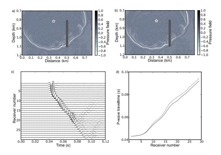
Fig. 13 Snapshot of the normalized pressure field at 90 ms before (a) and after the injection (b). The source and the vertical array of receivers are represented by the red star and vertical line, respectively. Panel (c) represents the normalized amplitude variation versus receiver number before and after injection (solid and dashed curves, respectively, and panel (d) shows the traveltime picks before and after injection (solid and dashed curves, respectively).
