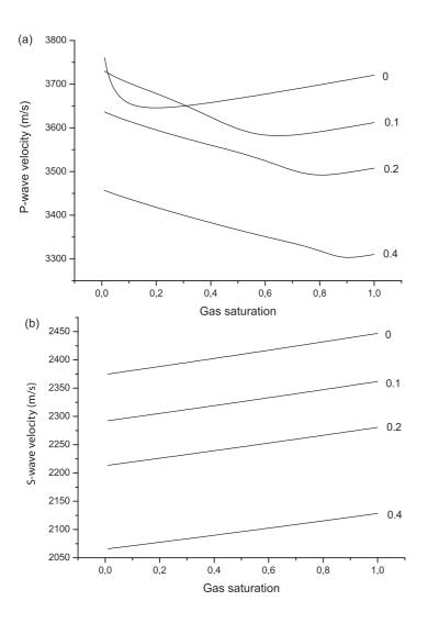
Fig. 2 P-wave (a) and S-wave (b) velocities as a function of gas saturation at 200 Hz. The numbers indicate the clay content.
