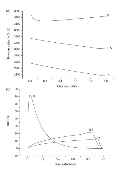
Fig. 5 P-wave velocity (a) and dissipation factor (b) as a function of the saturation for 0, 50 and 100 % clay content. The frequency is 200 Hz.
