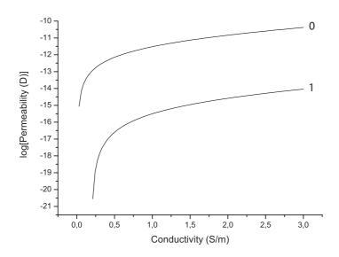
Fig. 6 Permeability as a function of conductivity for C=0 (clean sandstone) and C=1 (shale) (-12 correspond to 1 D).
