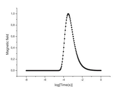
Fig. 8 Comparison between numerical and analytical solutions (normalized) at  $(x, z) = (50,50) \text{ m} (r \approx 70 \text{ m})$  from the source location (center of the mesh). The solid line corresponds to the analytical solution, obtained from equation (41).
