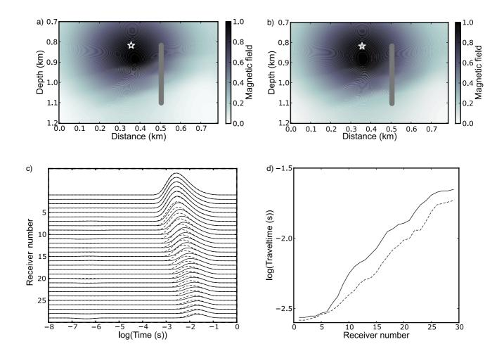
Fig. 12 Snapshots of the normalized magnetic field at 20 ms before (a) and after (b)  $CO_2$  injection. The source and the vertical array of receivers are represented by the star and vertical line, respectively. Panel (c) represents the normalized amplitude variation versus receiver number before and after injection (solid and dashed curves, respectively, and panel (d) shows the traveltime picks before and after injection (solid and dashed curves, respectively).
