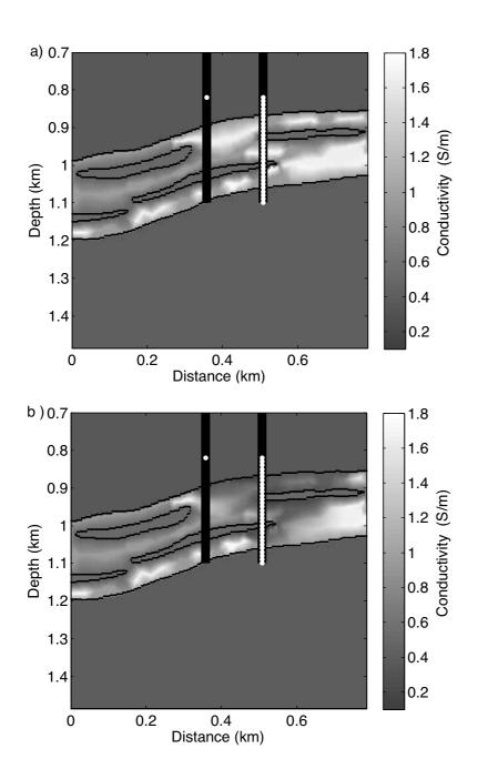
Fig. 10 Conductivity before (a) and after (b)  $CO_2$  injection.
