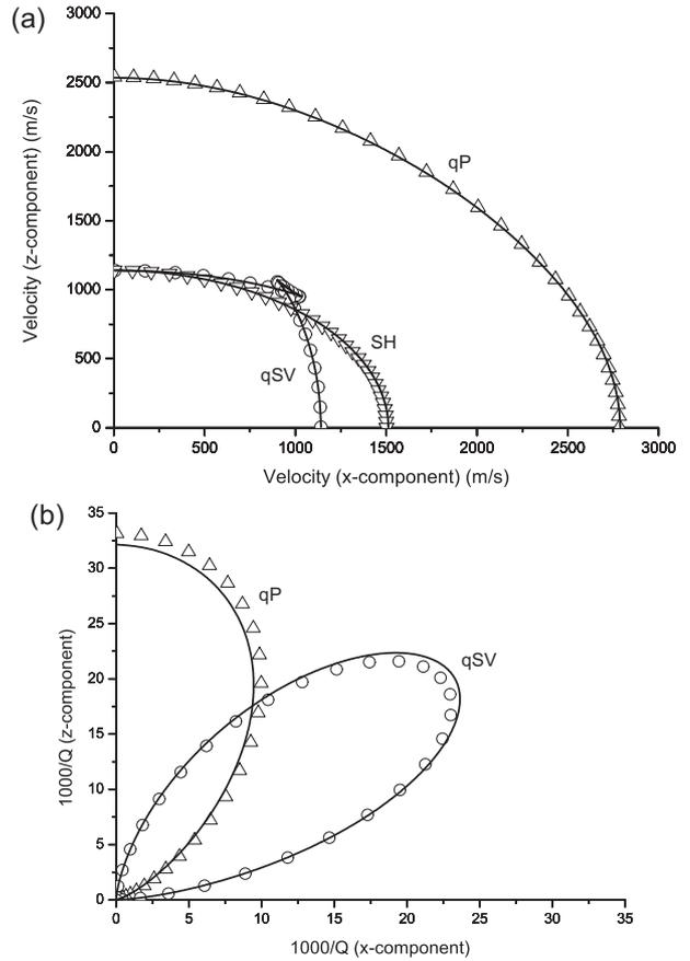
**Figure 5.** Polar representation of the energy velocity (a) and dissipation factor  $[(1000/Q)(\sin \theta, \cos \theta)]$  (b) corresponding to a frequency of 50 Hz. The medium consists of a sequence of mudstone and water-saturated sandstone layers of 5 cm and 1 cm, respectively (see Figure 4).
