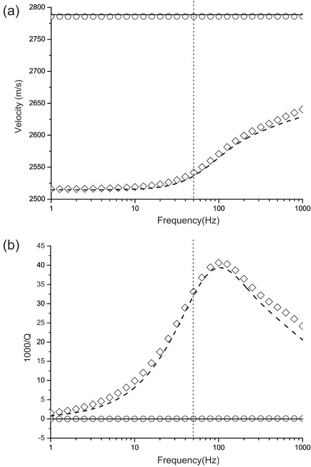
**Figure 4.** P-wave phase velocity (a) and dissipation factor (b) as a function of frequency in the directions parallel (circles and solid line) and perpendicular (diamonds and dashed line) to the layering plane. The symbols correspond to the FE experiments. The vertical line indicates the frequency (50 Hz) used for the polar plots. The medium consists of a sequence of mudstone and water-saturated sandstone layers of 5 cm and 1 cm, respectively.
