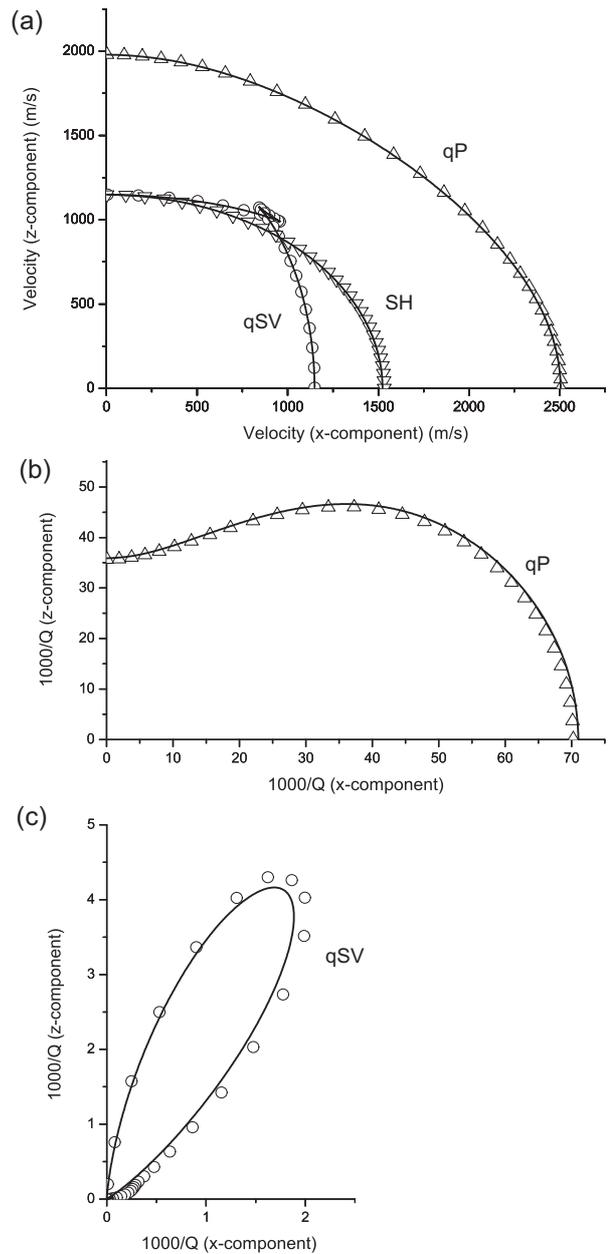
**Figure 7.** Polar representation of the energy velocity (a) and dissipation factors (b and c) corresponding to a frequency of 50 Hz. The medium consist of a sequence of mudstone and CO<sub>2</sub>-saturated sandstone layers with thicknesses of 5 cm and 1 cm, respectively (see Figure 6).
