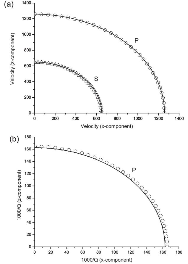
**Figure 3.** Polar representation of the energy velocity (a) and quality factor (b) corresponding to a frequency of 50 Hz. The medium consist of a sequence of gas and brine saturated thin sandstone layers. The gas saturation is 50 % ( $d_1 = d_2 = 30$  cm) (see Figure 1).
