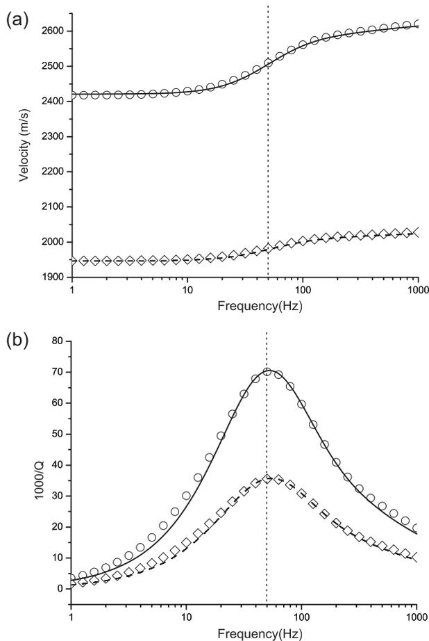
**Figure 6.** P-wave phase velocity (a) and dissipation factor (b) as a function of frequency in the directions parallel (circles and solid line) and perpendicular (diamonds and dashed line) to the layering plane. The symbols correspond to the FE experiments. The vertical dashed line indicates the frequency (50 Hz) used for the polar plots. The medium consist of a sequence of mudstone and CO<sub>2</sub>-saturated sandstone layers with thicknesses of 5 cm and 1 cm, respectively.
