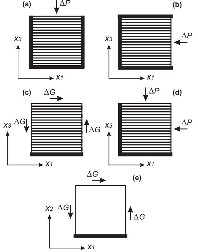
**Figure 1.** Oscillatory tests performed to obtain  $p_{33}$  (a),  $p_{11}$  (b),  $p_{55}$  (c),  $p_{13}$  (d) and  $p_{66}$  (e). The orientation of the layers and the directions of the applied stresses are indicated. The thick black lines at the edges indicate rigid boundary conditions (zero displacements).
